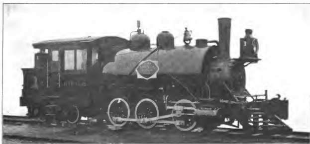
Fig. 18. Six-Coupled (0-6-4) Tank Locomotive. Built by the American Locomotive Co. for the Murphy Lumber Co. Cylinders 13 in. x 18 in., Working Steam Pressure 150 lbs. per sq. in., Heating Surface 723 sq. ft., Diameter of Drivers 38 in., Weight on Drivers 56,200 lbs., Total Weight 69,400 lbs.
